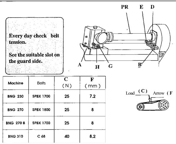
Loosen bolts (A, no. 4) and (B, no. 1) which fasten transmission to shredder frame. Loosen adjusting screw counternuts (H and D).
