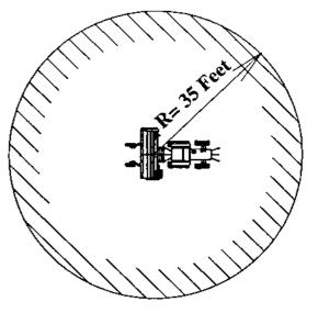
**BE PARTICULARLY CAREFUL WHEN YOU WORK ON RISES OR DITCHES.** THE UNEVEN GROUND CAN MAKE THE GUARDS TEMPORARILY INEFFICIENT AND ALLOW THE PROJECTION OF STONES OR FRAGMENTS IN A WIDE RANGE
