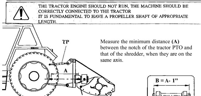
Measure the distance of the propeller shaft, in the position of <u>minimum</u> extension (all closed).
