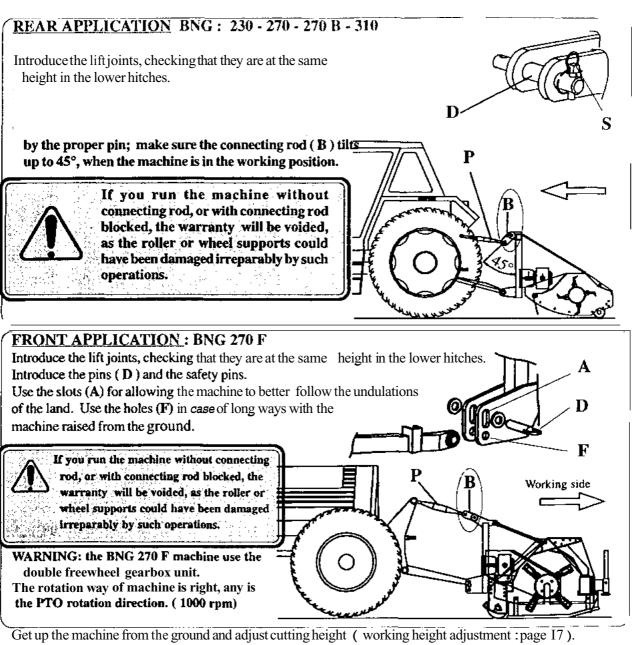
Get up the machine from the ground and adjust cutting height (working height adjustment : page 17). Raise foot and secure it.
