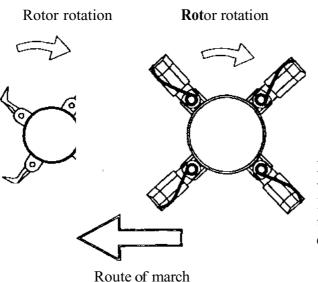
If the machine is equipped with Y blades with ventilating vanes, consider vane weight too. If ventilating vanes are fitted, make sure that their assembly was performed correctly, i.e. correct direction. (See the drawing).
