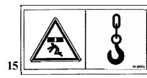
INDICATION OF THE HITCHING POINTS FOR MACHINE HOISTING
