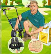
Border control is achieved by pushing the border control slider across (as in the picture below), you can shut off one side of the spreader. This helps save patio paths and flower borders from the spread of material where it's not required.
